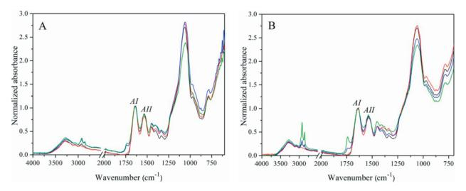
Fig. 8. Normalized FTIR spectra (Amide I) of photographic images of fields P1 (A) and P8 (B) for photographic paper N 112 (untreated sample – black line, sample after plasma treatment for 10 min – red line, untreated sample aged in Q-SUN for five days – blue line, sample after plasma treatment for 10 min and then aged in Q-SUN for five days – green line.
