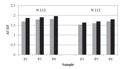
**Fig. 5.** Graphical representation of calculated ratios of Amide I (*AI*)/Amide II (*AII*) (untreated samples – gray, samples after 10 min of plasma treatment – black) for the selected fields P1, P5 and P8.
