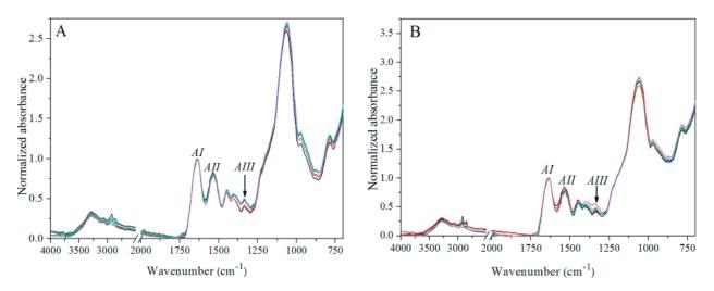
Fig. 4. Normalized FTIR spectra (Amide I) of photographic images of fields P1(A) and P8 (B) on photographic paper N 112 and their changes after plasma treatment (untreated samples – black line and samples after 30 seconds of plasma treatment – red line, 1 min – blue line, 3 min – green line, 5 min – azure line and 10 min – pink line).
