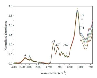
Fig. 2. Normalized FTIR spectrum (Amide I) of photographic image with different optical density D on photo paper N 112, D of individual areas is shown in Table 1 (P1 – black, P2 – orange, P3 – dark yellow, P4 – purple, P5 – green, P6 – blue, P7 – red, P8 – light green).
