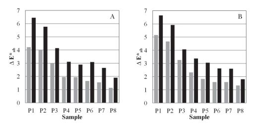
**Fig. 7.** Total color difference  $\Delta E^*_{ab}$  after aging for one day (gray columns) and for five days (black columns) for untreated (A) and plasma treated photographic paper (B) N 112.
