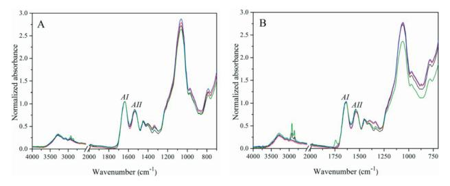
**Fig. 6.** Normalized FTIR spectra (Amide I) of photographic images of fields P1(A) and P8 (B) on N 112 photographic paper (untreated sample – black line, samples after plasma treatment, spectra of which were measured immediately after plasma treatment – red line, two days after plasma treatment – blue line and seven days after plasma treatment – green line).
