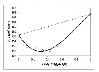
**Fig. 2.** Molar volume of the hypothetical liquid phase at 0 °C; (full line): calculated; (dotted line): ideal behavior (additivity of molar volumes).
