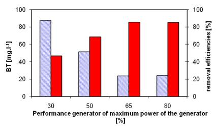
**Fig. 6.** Ozone generator impact on BT removal efficiency ■ and concentration of BT ■.
