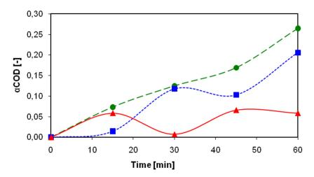
**Fig. 5.** Time dependencies of individual COD portions:  $aCOD_{axi} \bullet, aCOD_{miner} \bullet, aCOD_{parcoxi} \blacktriangle$ .
