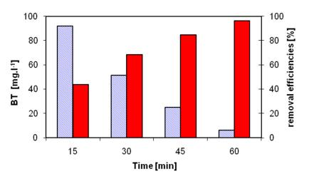
**Fig. 3.** Ozonation time impact on BT removal efficiency ■ and concentration of BT ■ in combined O3/ZEO process.
