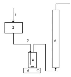
Fig. 1. Laboratory ozonation reactor.
