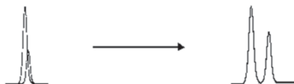
Fig. 1. Heart cutting for improved resolution. Overloading of peaks after separation in the first dimension (left) and resolved peaks after separation in the second dimension (right) on column with another polarity.
