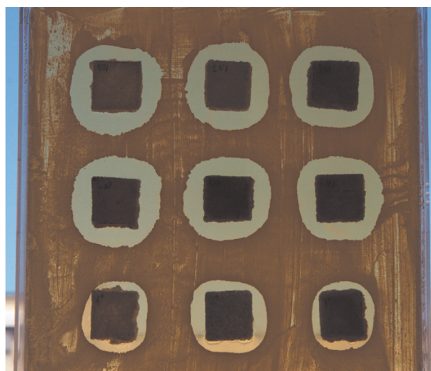
Fig. 6. Antimicrobial activity determination in direct contact with samples of chosen packaging materials with immobilized nisin.
