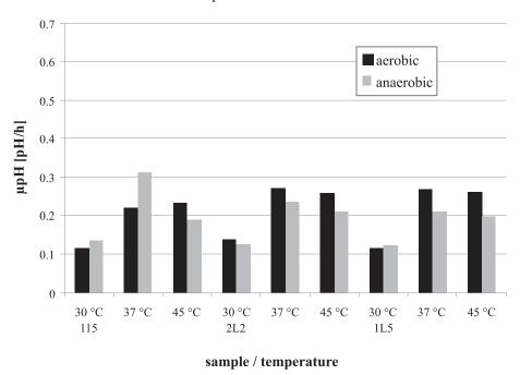
Fig. 6. Specific rates of pH decrease during 48 hour of cultivation.
