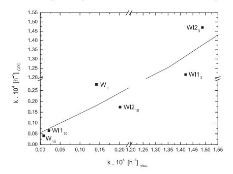
**Fig. 5.** Dependence of the rate constants of GPC on the rate constants of viscometry; paper Whatman No. 1 (W), model systems (W11, W12), pH 3 and pH 10.
