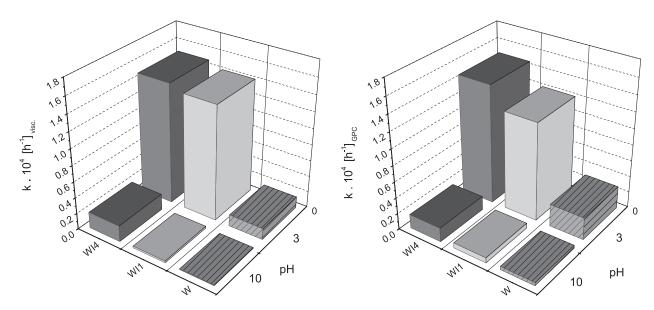
Fig. 3. The rate constants of degradation, viscometry; paper Whatman No. 1 (W), model systems (WI1, WI2), pH 3 and pH 10.
