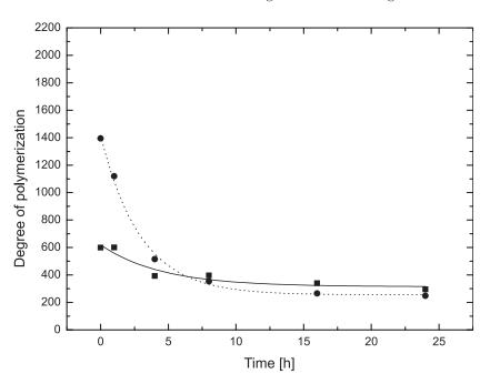
**Fig. 1.** Degradation curves (degrees of polymerization determined viscometrically and from GPC data); model system W11 – Whatman; iron-gall ink Fe(II):gallic acid = 0.25; pH 3, (GPC: solid squares, solid line; viscometry: solid circles, dot line).
