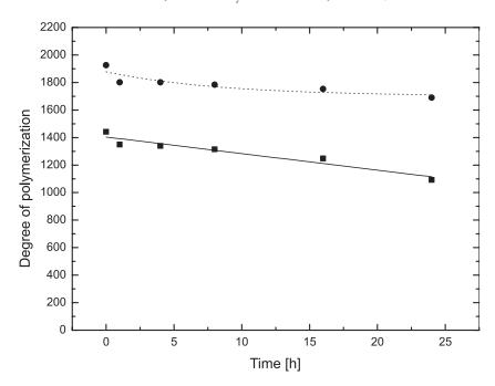
**Fig. 2.** Degradation curves (degrees of polymerization determined viscometrically and from GPC data); model system WI1 – Whatman; iron-gall ink Fe(II):gallic acid = 0.25; pH 10, ((GPC: solid squares, solid line; viscometry: solid circles, dot line).
