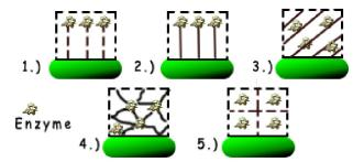
**Fig. 5.** Methods used for immobilization of enzymes and other bioreceptors in biosensors. 1.) Adsorption, 2.) Covalent binding, 3.) Matrix entrapment, 4.) Cross-linking, 5.) Encapsulation.
