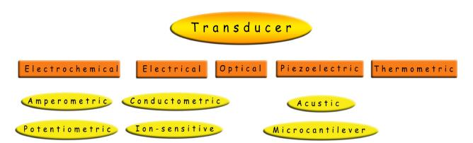
Fig. 4. Classification of transducers used in biosensors.
