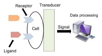
Fig. 3. Scheme of cell-based biosensor.
