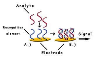
**Fig. 2.** General DNA biosensor scheme. Target DNA is captured at the recognition layer (A), and the resulting hybridization is transduced into a measurable electronic signal (B).
