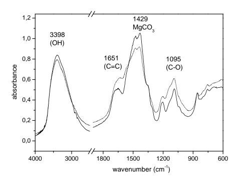
Fig. 11. FTIR spectra of iron gall ink with MMMK in pellet. Black line: no ageing, dot line: aged 3 days
