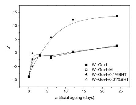
Fig. 8. The effect of accelerated wet ageing at 80°C, 50% RH on the change in the chromatic coordinate b\* for the ink samples
