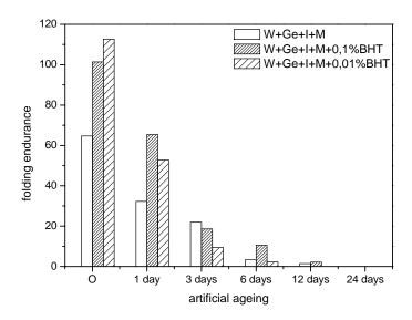
Fig. 2. Dependence of the number of folding endurance on the ageing time for wet ageing at 80°C, 50% RH for ink samples
