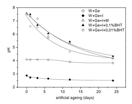
Fig. 4. Dependence of the pH on the ageing time for wet ageing at 80°C, 50% RH for ink samples
