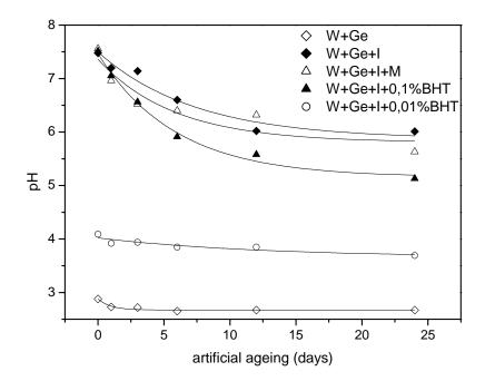
Fig. 5. Dependence of the pH on the ageing time for dry ageing at 105°C for ink samples
