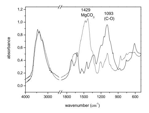
Fig. 10. FTIR spectra of iron gall ink (black line) and iron gall ink with MMMK (dot line) in pellet.
