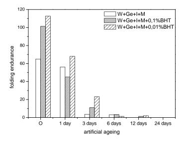
Fig. 3. Dependence of the number of folding endurance on the ageing time for dry ageing at 105°C for ink samples
