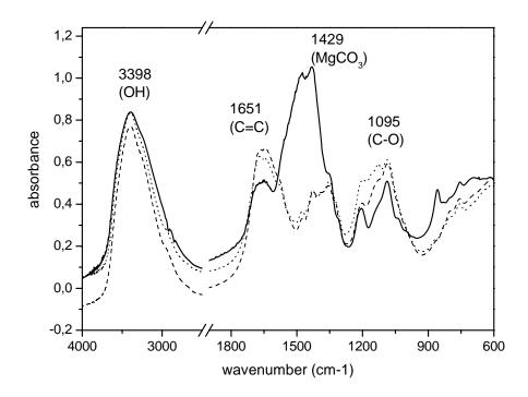
Fig. 12. FTIR spectra of iron gall ink with MMMK in pellet. Black line: no ageing, dot line: aged 12 days, dash line: aged 24 days
