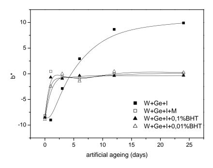
Fig. 9. The effect of accelerated dry ageing at 105°C RH on the change in the chromatic coordinate b\* for samples with applied ink
