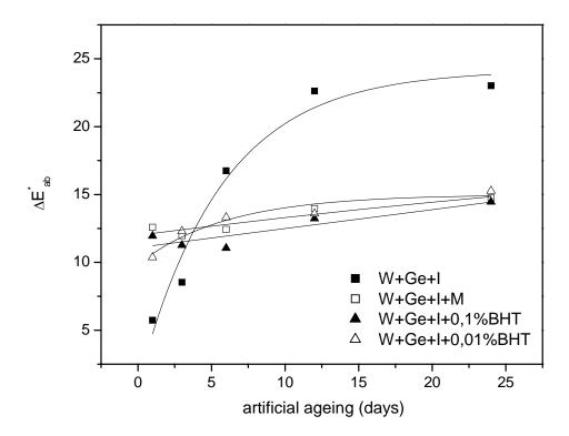
Fig. 6. Total colour difference in wet ageing at 80°C, 50% RH for samples with applied ink
