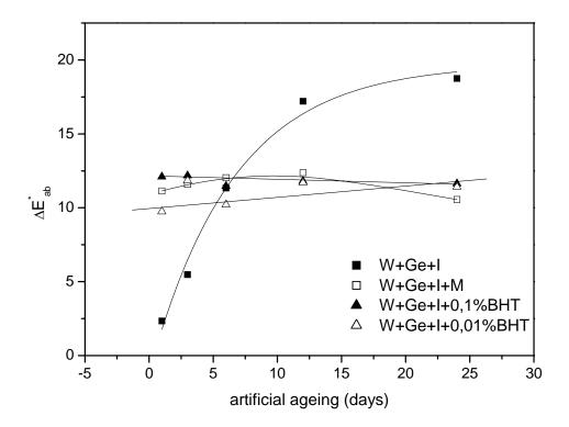
Fig. 7. Total colour difference in dry ageing at 105°C for ink samples
