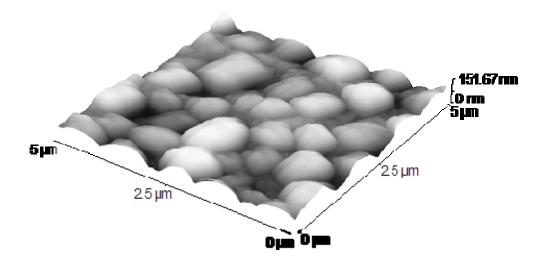
Fig.6 AFM image of the 5s plasma treated film, RSM= 24nm
