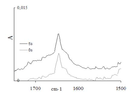
Fig.7 ATR-FTIR spectrum of untreated (0s) and plasma treated (5s) PP films
