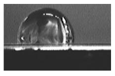
Fig.1 A drop of water on the PP film **before** treatment
