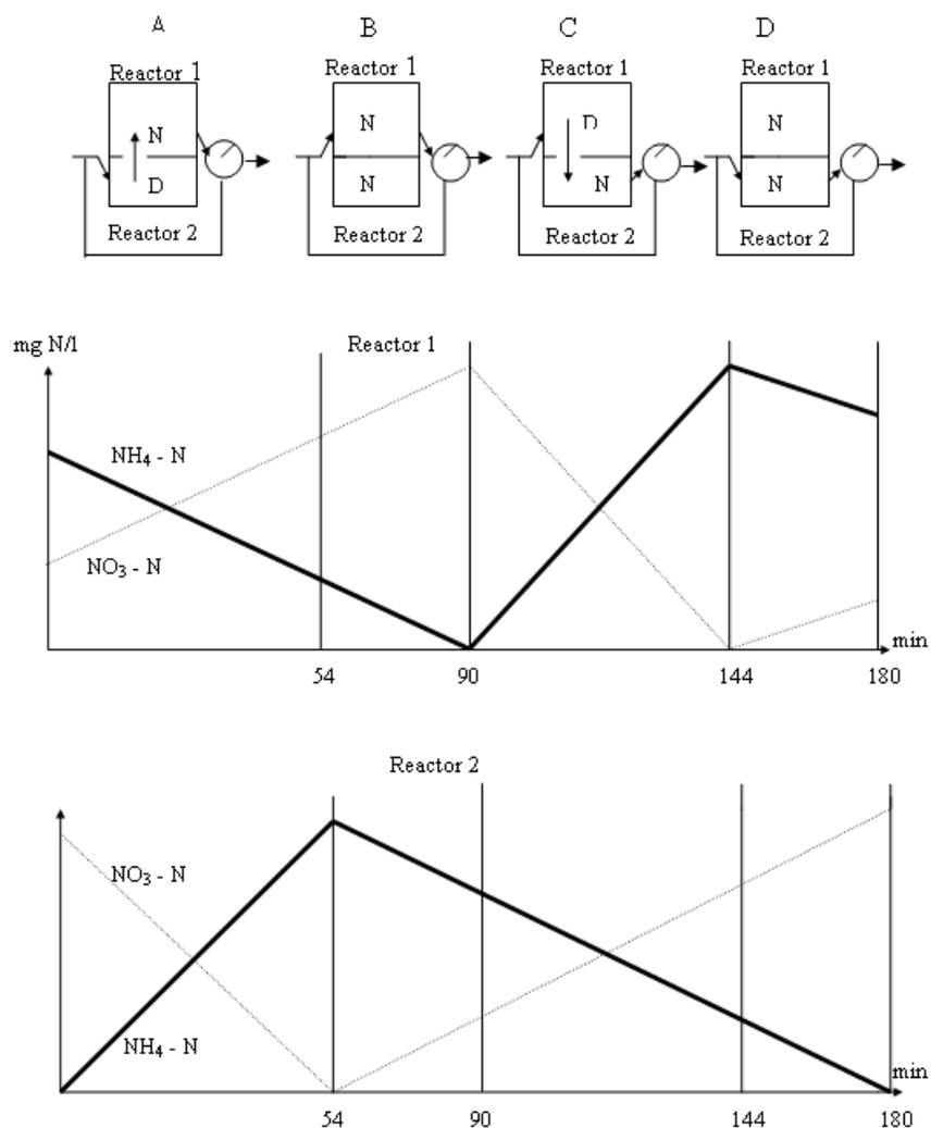
Fig. 1. Scheme of alternating denitrification cycle
