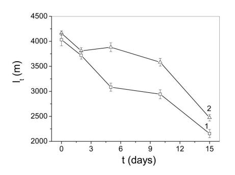
Fig.1. Effect of ageing time (t, days) on breaking length  $(l_t, m)$ : 1 – non - treated newsprint paper, 2 - newsprint paper treated by carbonated magnesium propylate dissolved in heptafluoropropane
