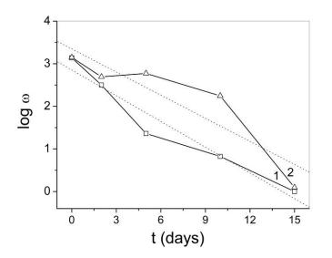
Fig.3. Effect of ageing time (t, days) on logarithm of folding endurance (ω, double folds): 1 - non-treated newsprint paper, 2 - newsprint paper treated by carbonated magnesium propylate dissolved in heptafluoropropane
