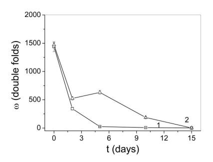
Fig.2. Effect of ageing time (t, days) on folding endurance ( $\omega$ , double folds): 1 nontreated newsprint paper, 2 - newsprint paper treated by carbonated magnesium propylate dissolved in heptafluoropropane
